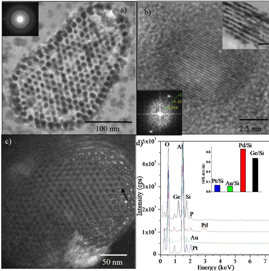
**Figure 3.** Pd-nanostructures prepared in non-calcined “columnar” mesostructured filaments. a) Plan-view TEM image (inset: corresponding SAED) and b) HRTEM image of one of the nanostructures shown in Figure 3a (inset: corresponding FFT and plan-view TEM image, scale bar 10 nm), and c) Ge-nanostructures in non-calcined columnar mesostructured filaments. d) Elemental analysis of the four different metal nanostructures discussed in this article.
