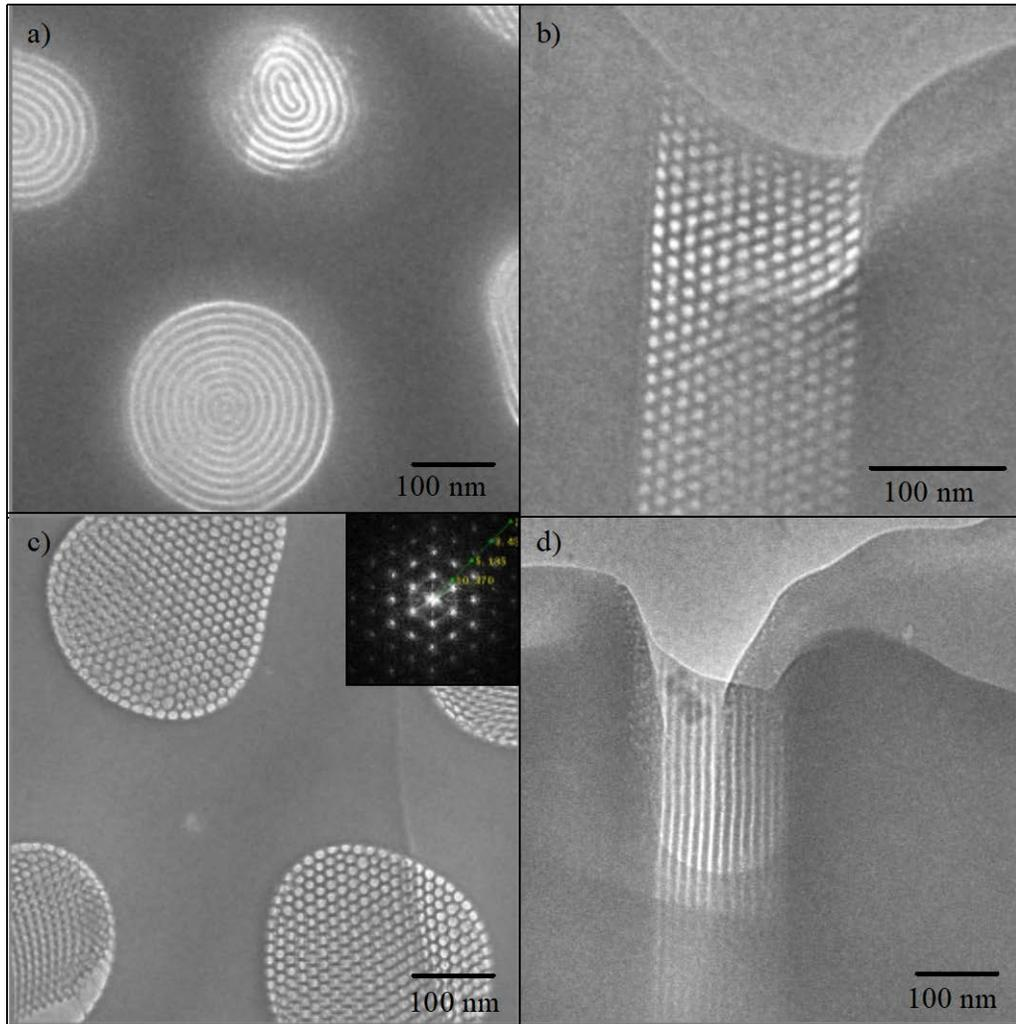
**Figure 1.** Mesophase morphologies observed in the AAM channels. Top: “Circular” mesophase structures, hexagonally ordered in the direction of the long axis of the filaments, showing a) plan- and b) side-view TEM images. Bottom: “columnar” mesophase structures, hexagonally ordered in the plane of the substrate, showing c) plan- and d) side-view TEM images (inset: FFT for one of the filaments shown in Figure 1c).
