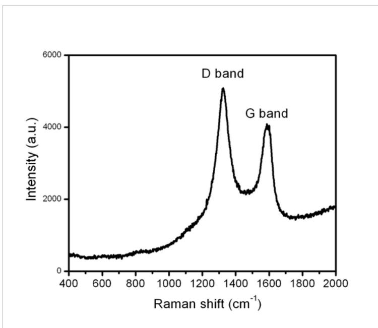
**Figure 6.** Raman spectrum of BCNTs after purification using 3 M HNO<sub>3</sub>.
