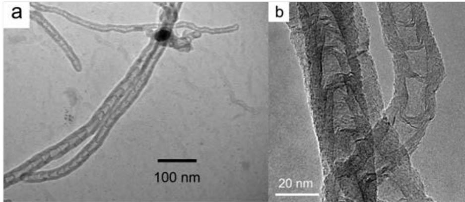
**Figure 4.** TEM images of bamboo-structured carbon nanotubes prepared by methane deposition over 10 wt% Cu and 5 wt% Mo at 850 °C for 1h.
