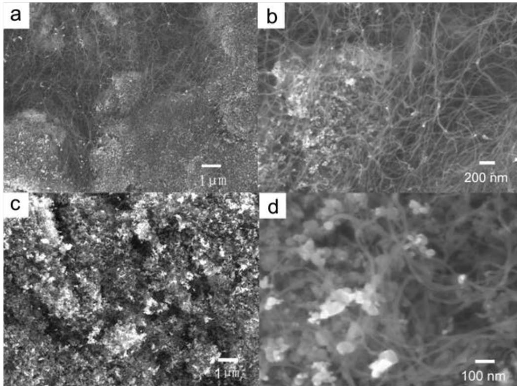
**Figure 3.** SEM images of carbon nanotubes prepared on (a, b) 5 wt% Cu and 5 wt% Mo and (c,d) 10 wt% Cu and 5 wt% Mo at 850 °C for 1 h.
