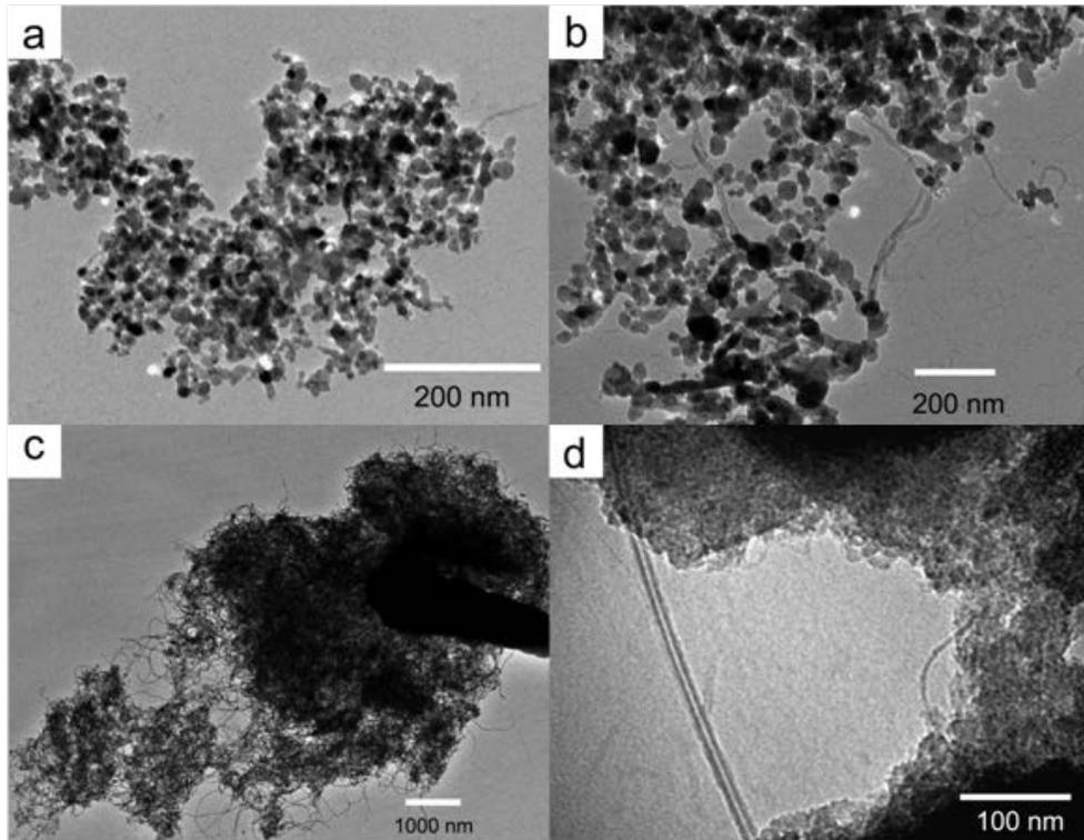
**Figure 2.** TEM images of carbon nanotubes prepared on: (a) 1 wt% Mo -10 wt% Cu/MgO, (b) 3 wt% Mo -10 wt% Cu/MgO, (c) 5 wt% Mo – 10 wt% Cu/MgO (d) 2wt% Cu - 5wt% Mo/MgO, at 850 °C for 1h.
