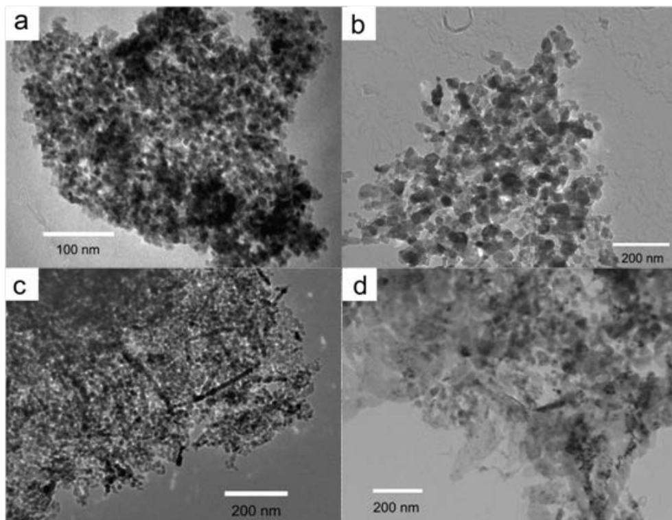
**Figure 1.** TEM images of catalysts after reaction with methane at 850 °C for 1 h: (a) 5 wt% Cu/MgO, (b) 10wt% Cu/MgO, (c) 5wt% Mo/MgO and (d) 10 wt% Mo/MgO.
