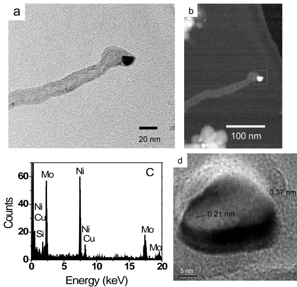
**Figure 5.** (a) Bright field and (b) dark field TEM images of a catalyst nanoparticle at the tip of a BCNT, (c) EDAX analysis of the catalyst nanoparticle and (d) HRTEM image of a catalyst nanoparticle (scale bar: 5 nm).
