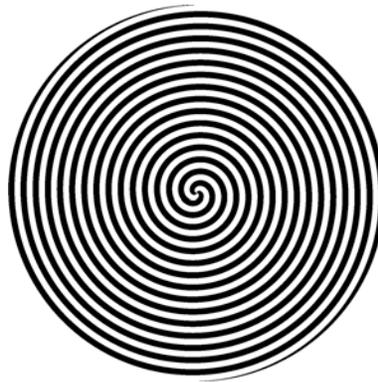
Fig. 1. A phase for fabricating a spiral axicon with  $m=2$ : the white spirals are phase  $\pi$ , and the black spirals are the phase of 0.
