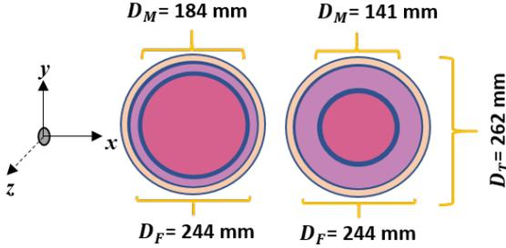
Fig. 1. Schematics of *Phantom 1* (left) and *Phantom 2* (right).
