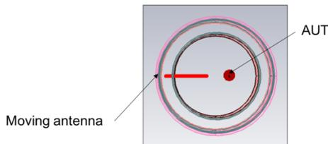
Fig. 2. Positioning of the antennas during measurements.
