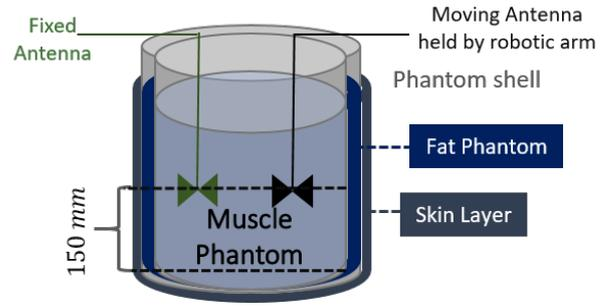
Fig. 3. Illustration of experimental setup showing tissue layers.
