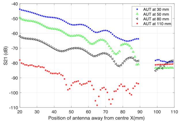
Fig. 4. Measured forward path gain  $|S_{21}|$  in *Phantom 1*.
