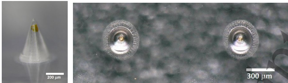
Figure 4. Left: example of reservoir-tipped microneedles after the filling procedure. Right: Top-down perspective of filled microneedles.
