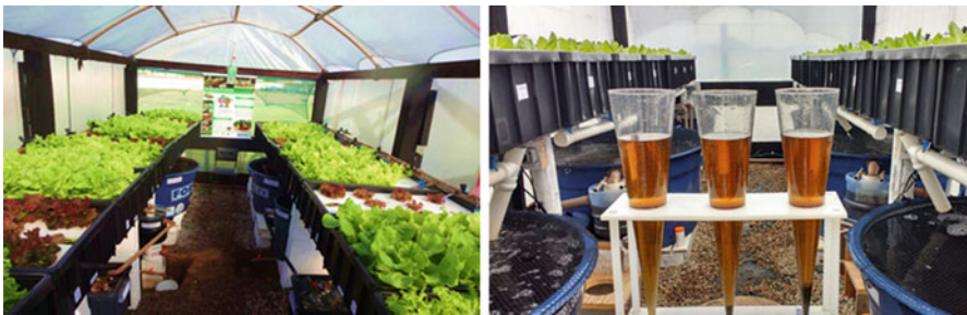
Fig. 12.6 Experimental aquaponics greenhouse comparing biofloc technology and RAS wastewater at Santa Catarina State University (UDESC), Brazil. (Source: Pinho et al. 2017)
