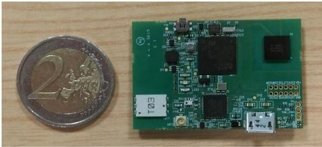
Fig. 1. Tyndall Wireless Inertial Measurement Unit (WIMU).
