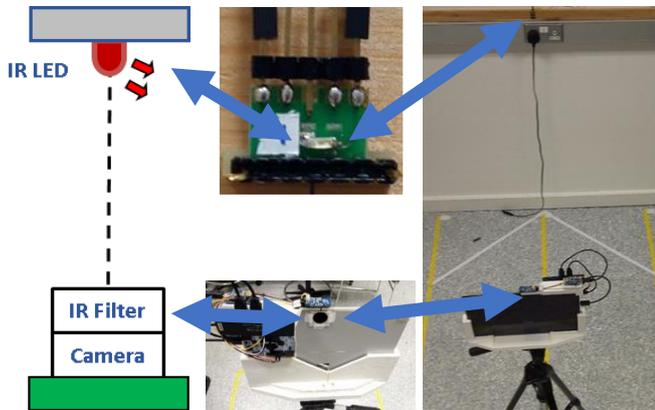
Fig. 3: Experimental Setup – Camera-IR Filter – IR LED
