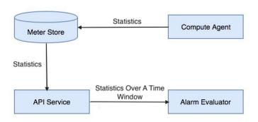
Figure 5.2: Ceilometer service components
