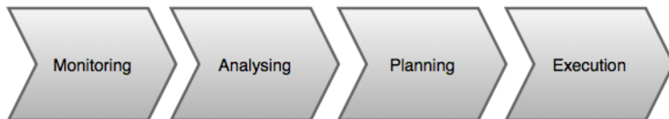
Figure 2.14: Different phases of the MAPE loop
