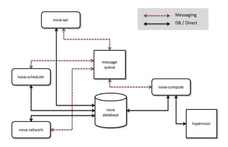
Figure 2.10: OpenStack Compute Architecture Overview
