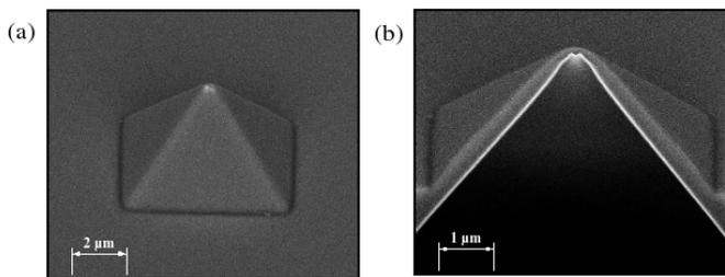
FIG. 4: (a) A secondary electron microscopy (SEM) image of the pyramidal tips used in the *Atom Pencil*. Panel (a) shows one of the pyramidal structures with a  $300\ \text{nm}$  hole in the apex of the tip. The base of the pyramid, as shown after the wet-etch process, is  $3.5\ \mu\text{m}$  on a side. The overall base of the pyramidal structure is  $22\ \mu\text{m}$  on a side. Panel (b) shows a focused ion beam (FIB) milled cross-section of the pyramidal tip aperture.
