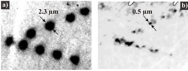
FIG. 3: Examples of structures consisting of a V-shaped stepped series of dots written with apertures of two different diameters: (a)  $1\ \mu\text{m}$ , (b)  $400\ \text{nm}$ . In (b) the distance aperture-substrate was well below  $200\ \mu\text{m}$  and the exposure time per dot was 180-200 s.
