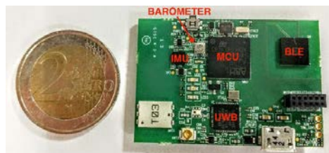
Fig. 2. Tyndall Wireless Inertial Measurement Unit (WIMU) [26].
