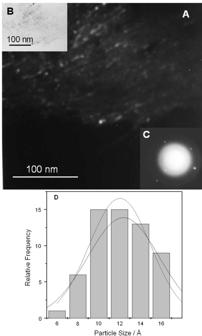
Fig. 3. Dark-field TEM image of the gold nanoparticles (Au-NPs) in acetone ([Au]:  $4 \times 10^{-3} \text{ mol dm}^{-3}$ ) (A). Bright-field TEM micrograph of randomly dispersed gold nanoparticles (B) and corresponding electron diffraction pattern (C). Histogram of Au-NPs size distribution. Gaussian fits are overlaid for comparison giving an average value of 1.2 nm for the nanoparticle diameter(D).
