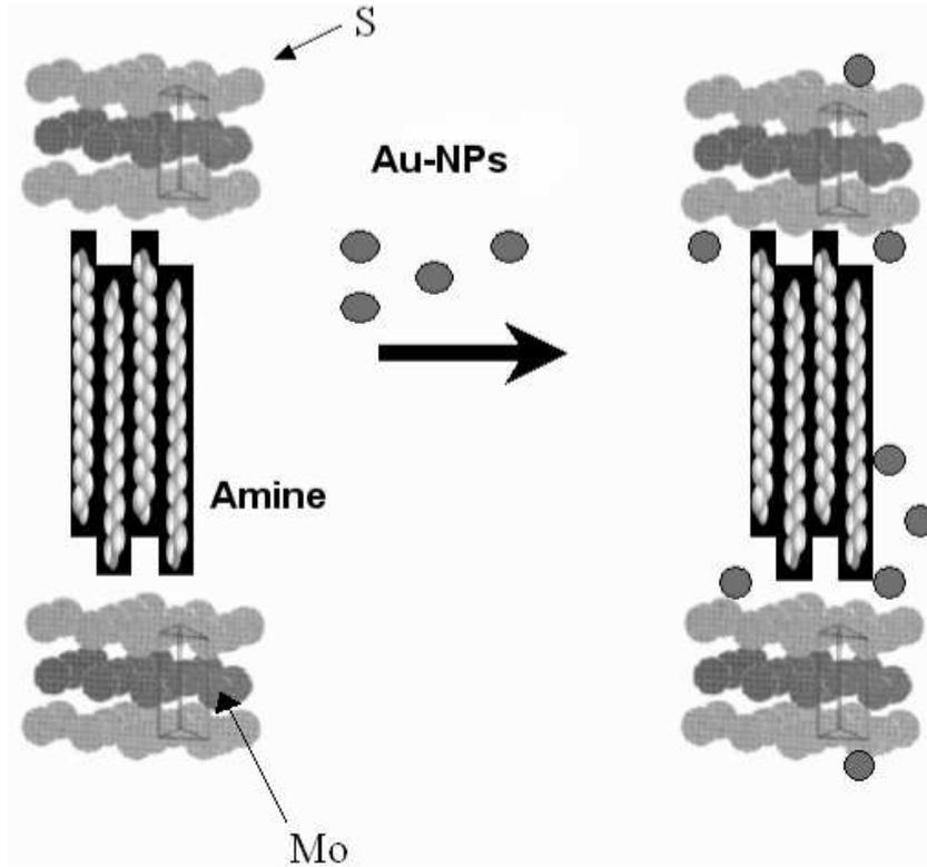
Fig. 6. Schematic representation of the functionalization of the  $\text{Li}_{0.1}\text{MoS}_2(\text{HDA})_2$  compound with gold nanoparticles and their position in the lamellar system. The  $\text{MoS}_2$  is represented in the 1T conformation [1].
