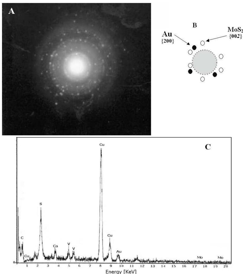
Fig. 5. (a) Electron diffraction pattern of the  $\text{Li}_{0.1}\text{MoS}_2(\text{HDA})_2$  compound after the functionalization with gold nanoparticles and (b) indexation of the contributions from  $\text{MoS}_2$  and  $\text{Au}\{111\}$ . (c) Energy dispersion spectroscopy analysis of the same compound.
