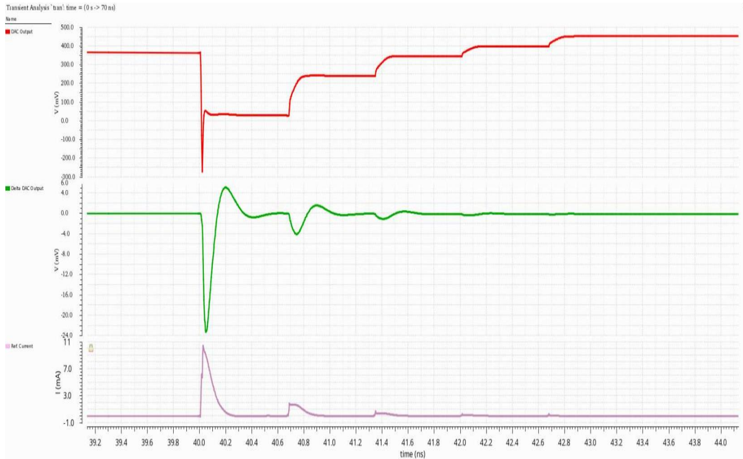
Figure 4.8 DAC step settling and difference between settling with ideal reference and buffer reference
