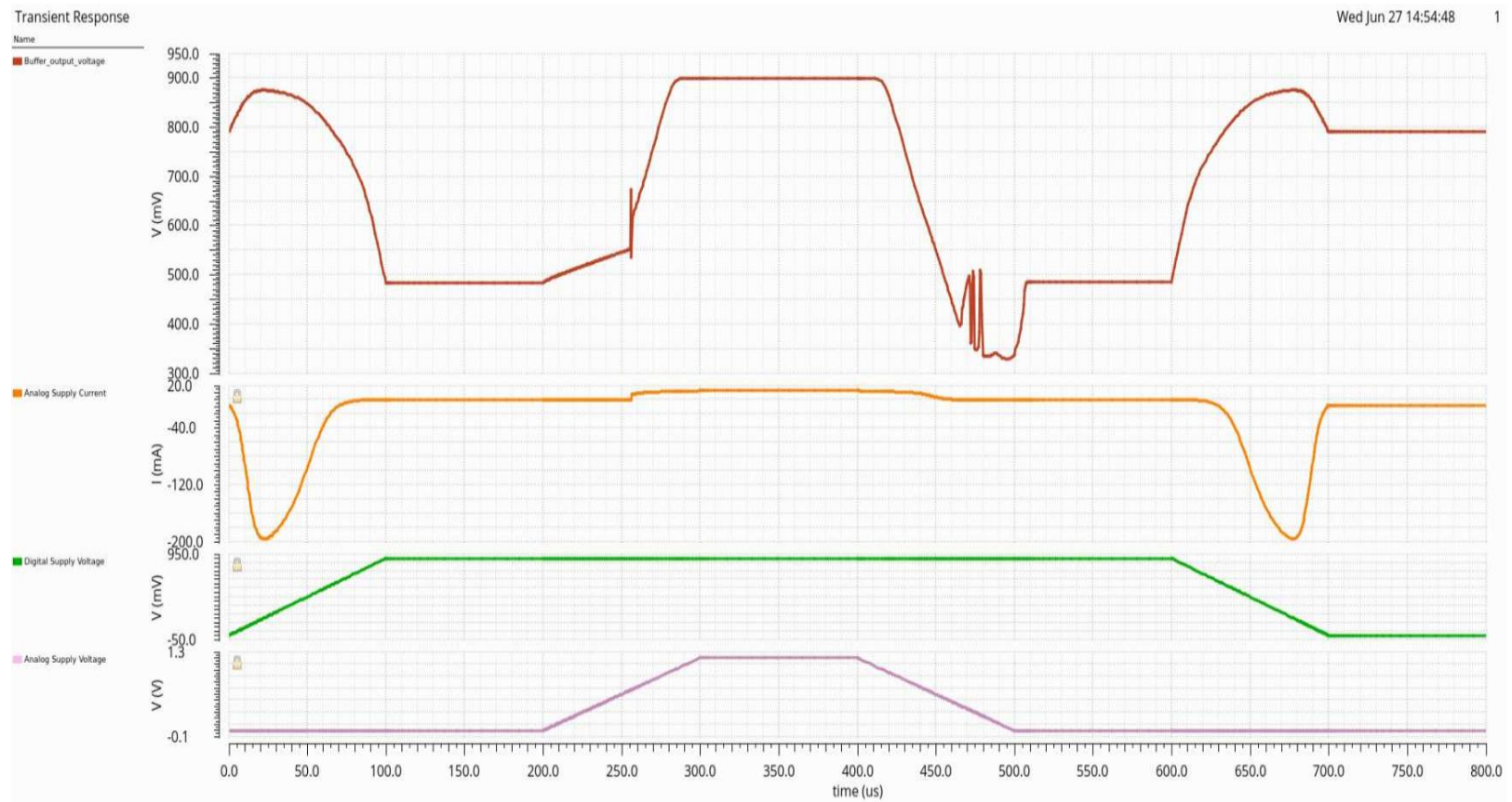
Figure 4.16 Power up/down of Analog & Digital Supplies
