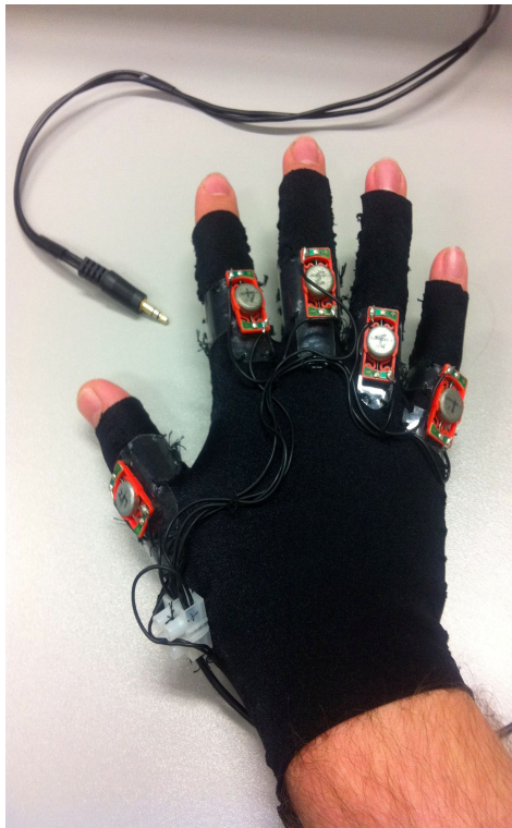
Figure 3.3: The Audio-Tactile glove [93].
