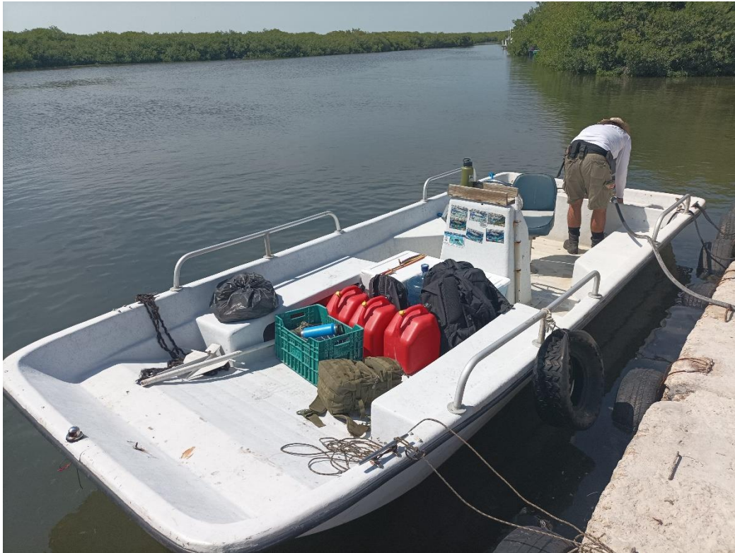
Figure A3.5: 19.6ft Carolina Skiff with a 40hp Yamaha four stroke outboard used for crocodile surveying. Source: Ciarán Ó Mordha.
