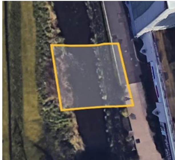
Fig.25: A 10 ×10 square representing a pixel size from a Sentinel 2 image. This shows three separate classes in one pixel, part of the river Bride, a non-woody and a built section, demonstrating the difficulty in accurately classifying the water class in Cork City. Source: Google Earth
