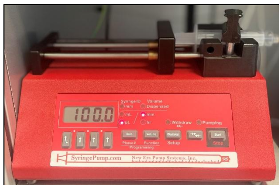
Figure 21: An image of the syringe pump used in the BioDep™ plasma system, located in TheraDep Ltd, Clonmel, Ireland.
