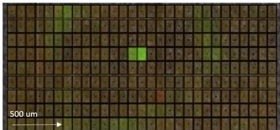
Figure 35: DUV map of everolimus coating deposited via wet deposition (no plasma, 0 V) onto a titanium disc, green indicates presence of drug while red indicates no drug present (500 points of 100 \mu\text{m} measured).
