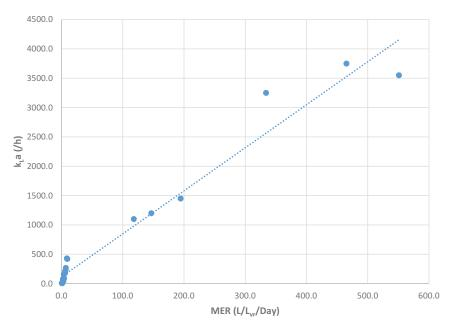
**Figure 13.** Comparison of MER vs  $k_L a$  data in literature.
