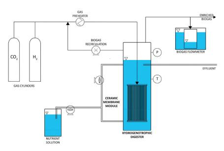
Figure 8. Diagram of a membrane bio-reactor experimental set-up.
