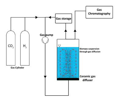
Figure 5. Modified CSTR with a ceramic diffuser base.
