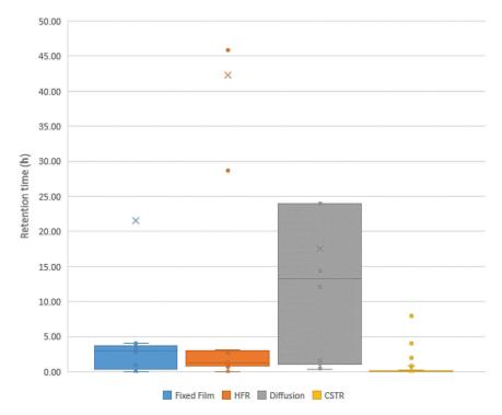
Figure 10. Comparison of retention times across reactor systems.
