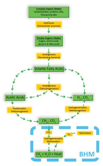
**Figure 3.** CH<sub>4</sub> formation through anaerobic digestion and biological hydrogen methanation.
