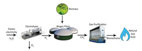
Figure 1. In-situ biological H<sub>2</sub> methanation schematic.
