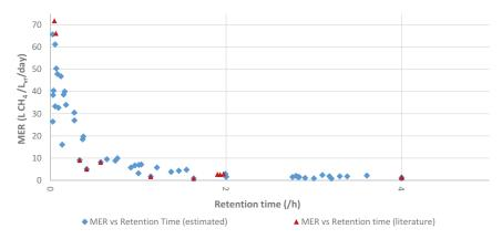
Figure 11.: Relationship between MER and retention times.
