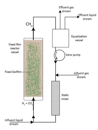
Figure 6. Fixed film/Anaerobic Filter and Soil packed reactor layout.
