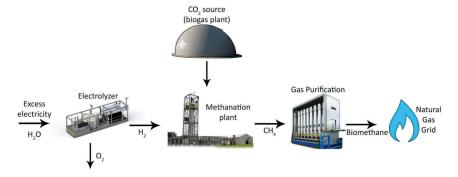
Figure 2. Ex-situ biological H<sub>2</sub> methanation schematic.
