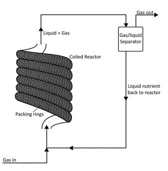
Figure 7. A novel BHM system using tubular reactor setup of narrow diameter pipe and packed fixed biofilm.
