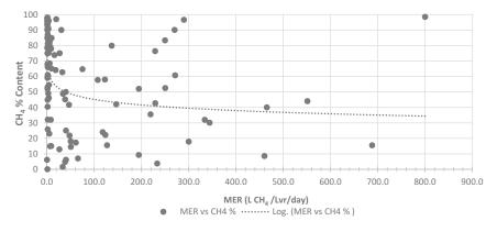
Figure 12.: Relationship between MER and CH<sub>4</sub>% content.
