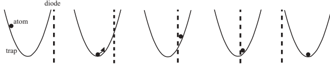
FIG. 1. Schematic representation of the process for a single atom: snapshots for different, increasing times (from left to right); the passing direction of the diode is from left to right.
