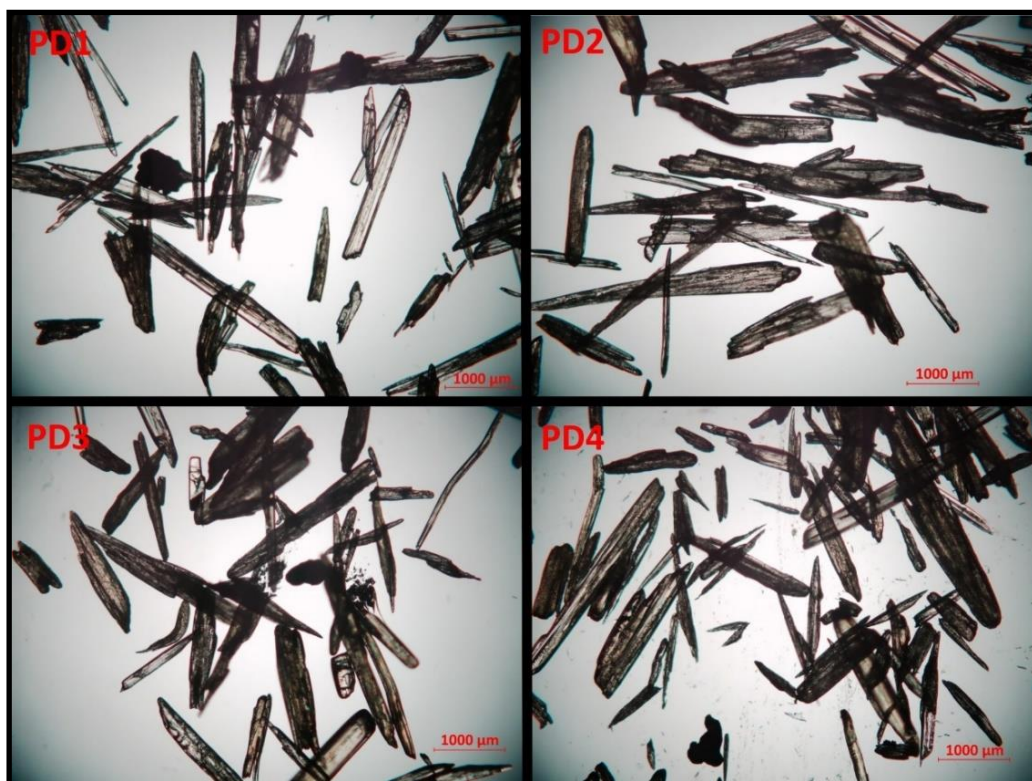
Fig S30. Microscope images (x40) of FFA crystals (containing ca. 2% t BuFA) after four partial dissolution stages, PD1 to PD4.
