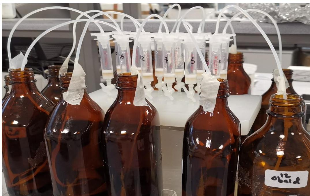
Figure 2-9: Samples undergoing SPE in the laboratory using a 12-position manifold.
