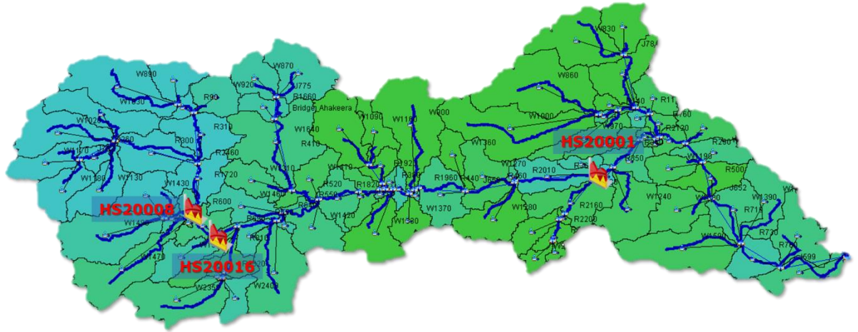
Figure 8.13. Control points (HS2008, HS20016 and HS2001) for calibration of Bandon HEC-HMS model.
