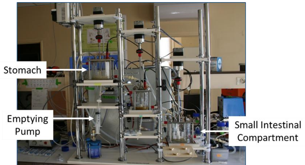
Figure 2 The DIDGI in vitro digestion system, STLO, INRAE, France. This is a multi-compartmental system, consisting of both gastric and small intestinal compartments. Food is automatically emptied from one stage of digestion to the next using emptying pumps.
