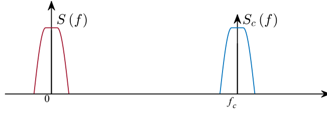
Figure 2–7. Illustration of the spectra of a baseband signal and its pass-band copy.
