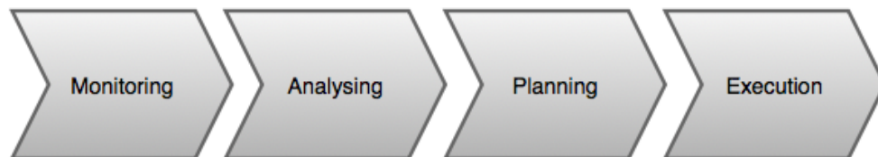
Figure 2.14: Different phases of the MAPE loop
