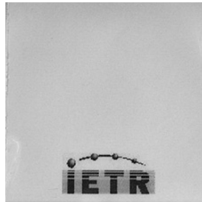
FIGURE 3. An ITO film on a printed paper demonstrating high transparency. (Reproduced from [26] with permission. Copyright © 2009 IET).
