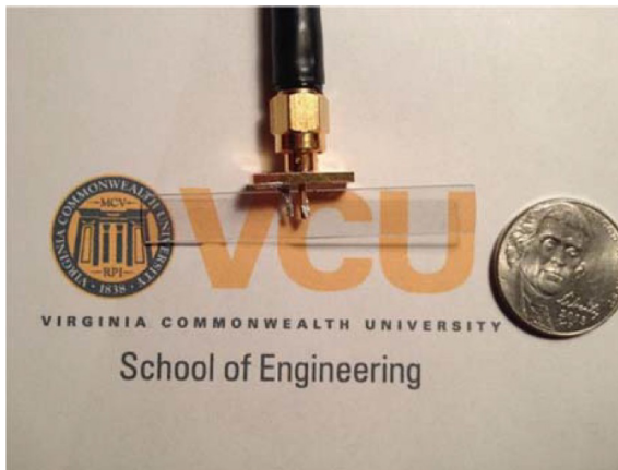
FIGURE 28. Fabricated transparent GZO dipole antenna. (Reproduced from [9] with permission. Copyright © 2017 Wiley Periodicals, Inc).
