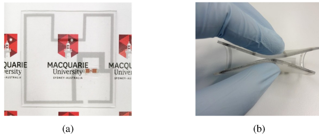
FIGURE 20. Photographs of the fabricated prototype of the RFID antenna made with VeilShield-PDMS composite: (a) unbent state, (b) bent state. (Reproduced from [72] with permission. Copyright © 2020 IEEE).
