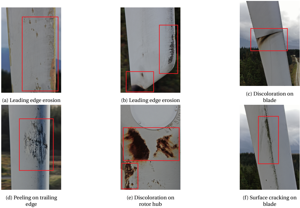
Figure 5.2: A subset of the RGB images acquired from the UAV with various types of damages boxed in red.
