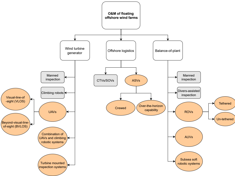
Figure 2.4: Research pertaining to robotics for O&M. rectangular areas (grayed): widely investigated. Elliptical areas (with filled color): possible research gaps.
