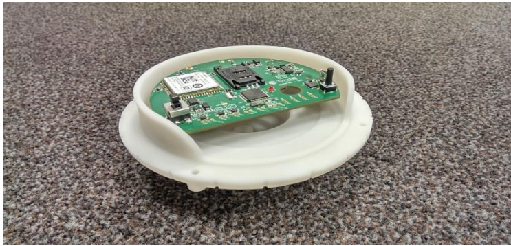
Figure 5. System Enclosure, lower half with PCB placed
