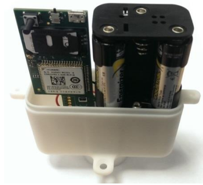
(b) The assembly of the board inside the enclosure.
