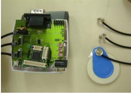
Figure 2. Wireless Patient Module with miniaturised Tyndall mote
