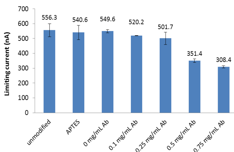
Figure 6.18: Reduction of limiting current calculated for the 10 \text{ }\mu\text{m} microband array according to surface functionalization.
