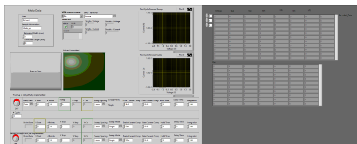
Figure D.5: Labview Front panel representation of Paramater analyser control software for determining the resistance of test structures.
