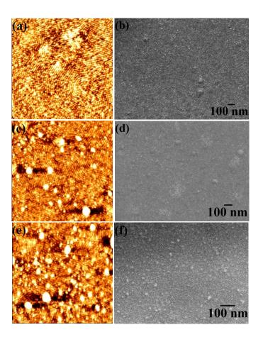
**Fig. 4** Surface morphology and topography of the iron oxide nanopatterns prepared with 1.8 wt% of iron nitrate-2 propanol solution stirred for different time of (a, b) 45 min (c, d) 1 h and (e, f) 1 h 30 min respectively.
