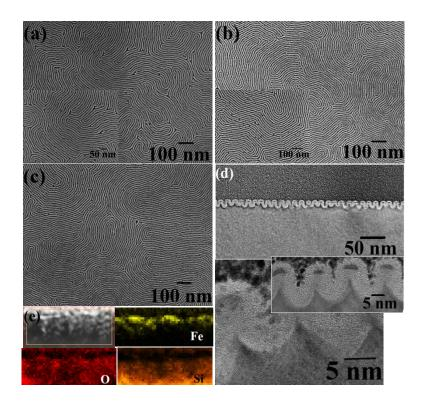
**Fig. 7** SEM images of Si nanowire arrays with iron oxide as a hard mask after (a) 30 sec (b) 45 sec and (c) 1 min Si etch respectively. (d) Cross sectional TEM and HRTEM images of Si nanowires with iron oxide at top. (e) elemental mapping of Fe, O and Si.
