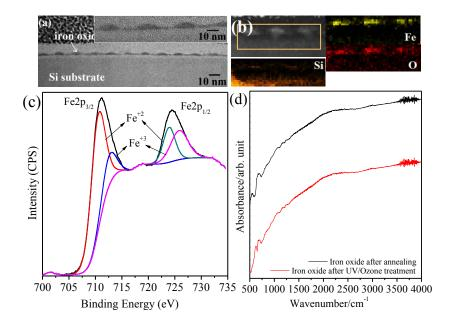
**Fig. 6** (a) Cross sectional TEM images of lamellar phase iron oxide nanowire arrays. (b) elemental mapping of Fe, O and Si. (c) Fe 2p spectra of iron oxide nanowires after UV/Ozone treatment (d) FTIR spectra of iron oxide nanowires after UV/Ozone treatment and further annealing.
