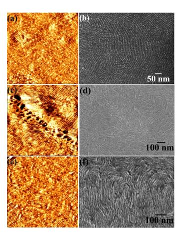
**Fig. 3** Surface morphology and topography of the iron oxide nanowires prepared with different concentrations of iron nitrate-2 propanol solution stirred for 30 min (a, b) 1.5 wt% (c, d) 2 wt% and (e, f) 2.2 wt% respectively.
