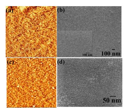
**Fig. 2** (a, c) AFM and (b, d) SEM images of iron oxide and nickel oxide nanowire arrays formed after UV/Ozone treatment respectively.
