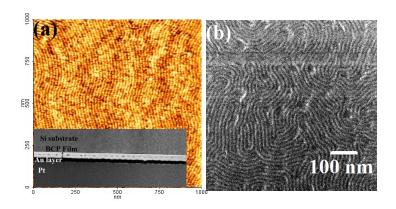
**Fig. 1** (a) Tapping mode AFM, (inset of a) Cross-sectional TEM and (b) SEM image of the surface morphology of the PS-b-PEO thin film following solvent annealing in toluene at 60° C for 30 min with the addition of 0.05 ml of LiCl-THF.
