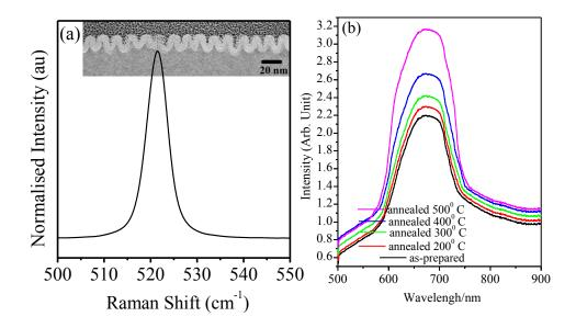
**Fig. 8** (a) Raman spectrum of Si nanowire arrays. (b) PL spectra of as-prepared Si nanowire arrays and annealed nanowires at different temperatures.
