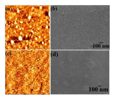
**Fig. 5** (a) AFM and (b) SEM images of iron oxide nanopatterns prepared with 1.8 wt% precursor dissolved in anhydrous ethanol stirred for 30 min. (c) AFM and (d) SEM images of iron oxide nanopatterns prepared with 1.8 wt% precursor dissolved in 2-propanol stirred for 30 min using LiCl-ethanol mediated BCP thin film.
