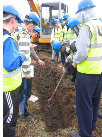
Figure 2 Trial pitting for geotechnical PBL
