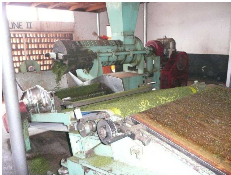
Figure 5: Drives in the fermentation section
