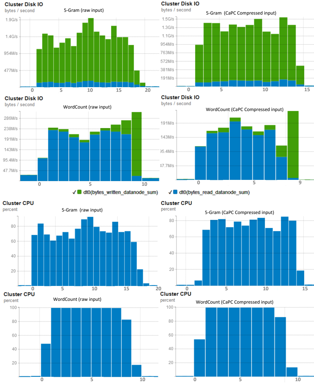
Figure 3.6: Statistics on Disk I/O and CPU utilization ( DataNodes ) for 5-Gram and WordCount jobs with original data and CaPC compressed data, respectively. (X-axis indicates job durations)
