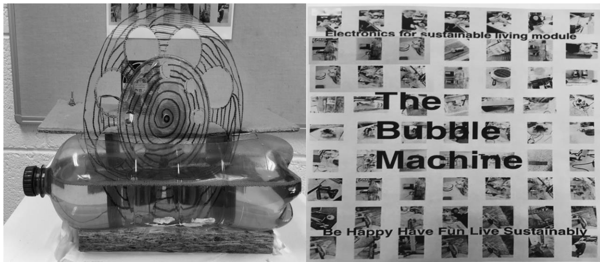
Figure 2. Bubble making machine using eco-friendly washing up liquid and dual motor system
