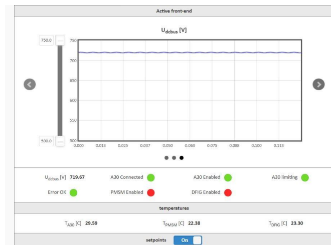
Figure 8: Voltage of the dc bus of the generator connected inverter showing some ripple
