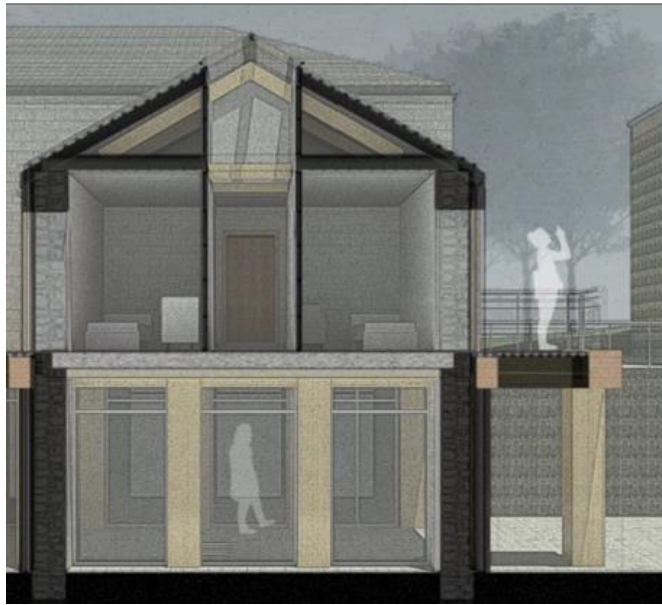
Figure 8: Enhancing circulation corridors by introducing building natural light through ridge glazing on the roof (Matthew Hurley, 2021)
