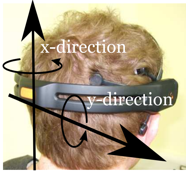
Figure 4.1: Emotiv EPOC headset: Gyroscope axes.
