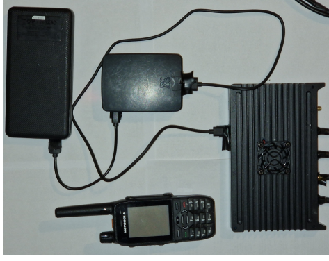
Fig. 2. Powerbank-powered Raspberry Pi 4 with the Kraken receiver, and Motorola handset.
