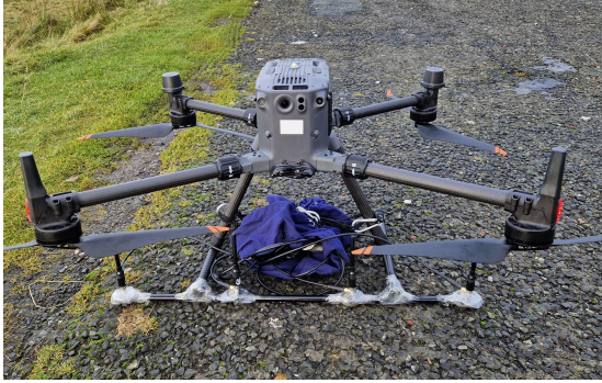
Fig. 3. DJI Matrice 350 UAV, with the dipole antenna ULA and electronic payload.
