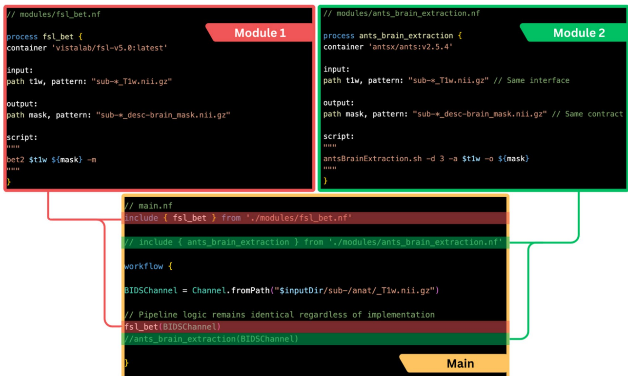
Fig. 3 Example Nextflow snippets demonstrating how different processes—FSL (red, fsl_bet.nf ) and ANTs (green, ants_brain_extraction.nf )—performing equivalent tasks through standardized
