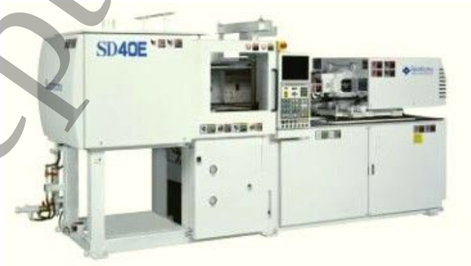
Figure 2. Sumitomo Disc 40E Disc Moulding Subsystem [44].
