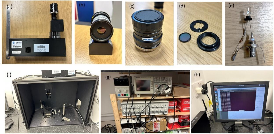
Figure 2.1: Components used to build the new wide-field Tpx3Cam imager. (a) Tpx3Cam coupled to Cricket, filter and lens; (b) Cricket adapter; (c) Lens; (d) C-mount and ring connectors, (d) LED; Imager setup covered in black box; Electronic connections of pulse generators, oscilloscope and power supply; (d) PC for collection of raw data.
