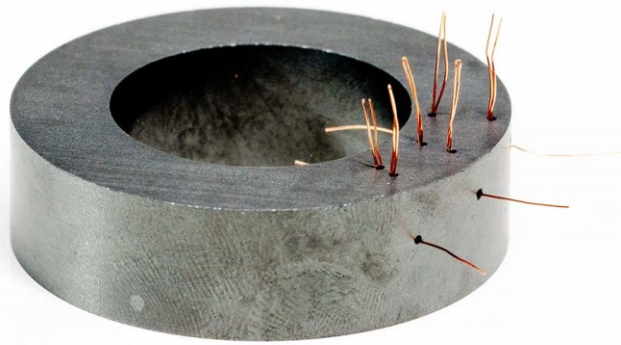
Figure 108. Tested core with sense winding.
