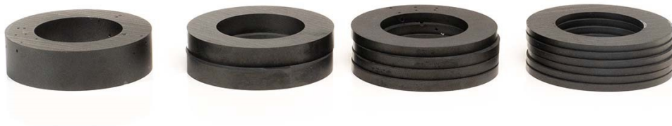
Figure 118. T50 cores to test lamination thickness impact on core performance.
