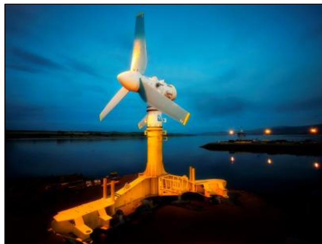
Figure 2-2: AR1500 tidal turbine supported on a steel tripod gravity-based foundation installed during the MeyGen project (Phase 1A). Source: (Rajgor, 2016)
