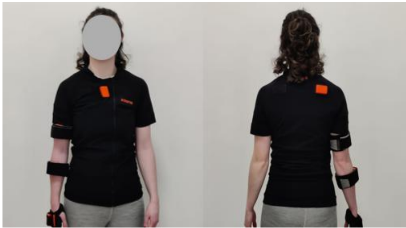
Figure 16: IMU placement on the shoulder, upper arm, forearm, hand and torso.
