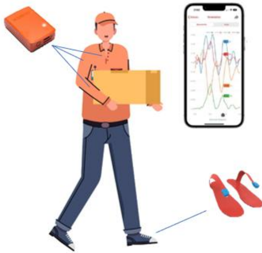
Figure 3: Fatigue forecasting system consisting of IMUs, pressure insoles and custom application
