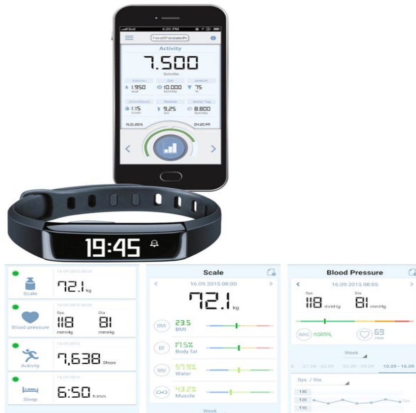
Figure 3.3 Activity Sensor linked by Bluetooth to Health-coach App on Mobile Phone Displayed image is the property of its rightful owner; adopted from: Sanitas HealthCoach App (Sanitas-online, 2021); adapted for illustration.
