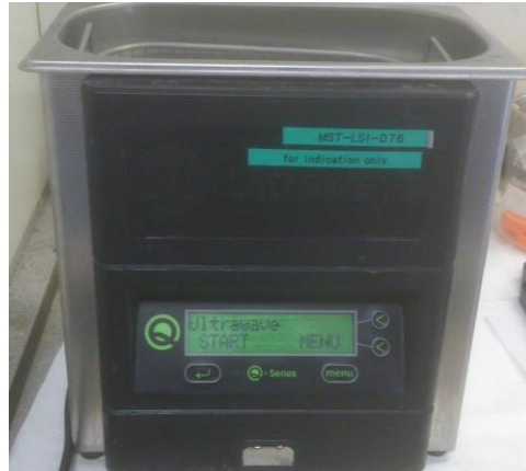
Figure 2.14: The Ultrawave QS3 ultrasonic water-bath used during the probe cleaning protocol.
