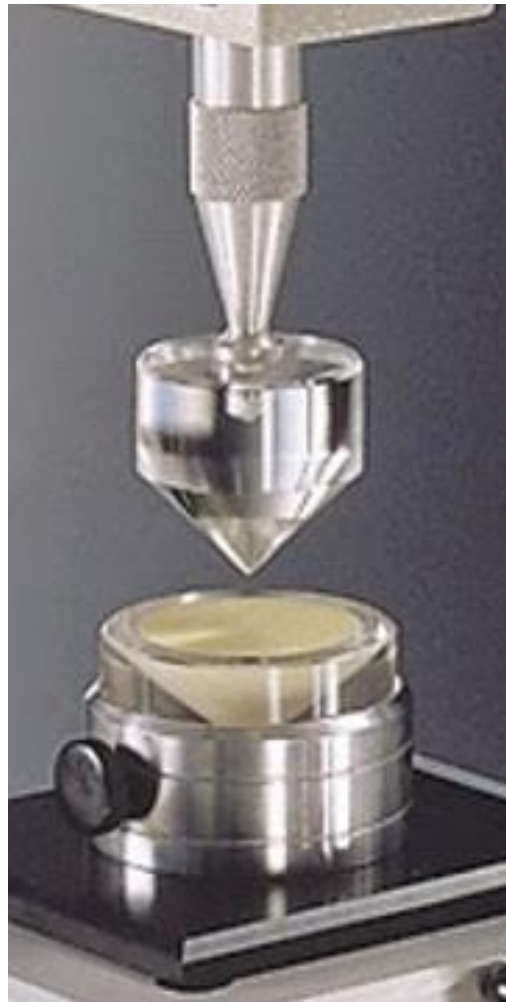
Figure 4.3. Conical spreadability probe used for spreadability analysis (Stable Micro Systems, 2025).
