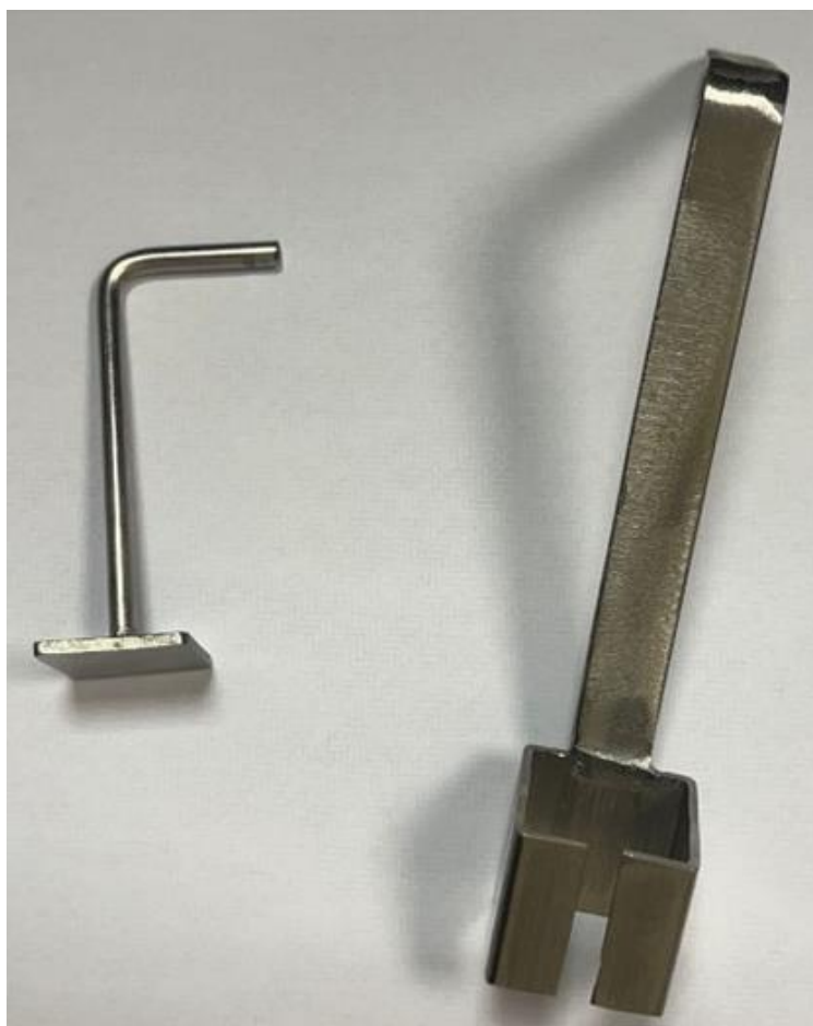
Figure 3.3. Custom-made metal cuber of dimensions 25mm x 25mm x 25mm (W x D x H) (Kerry Ingredients, Listowel County Kerry)
