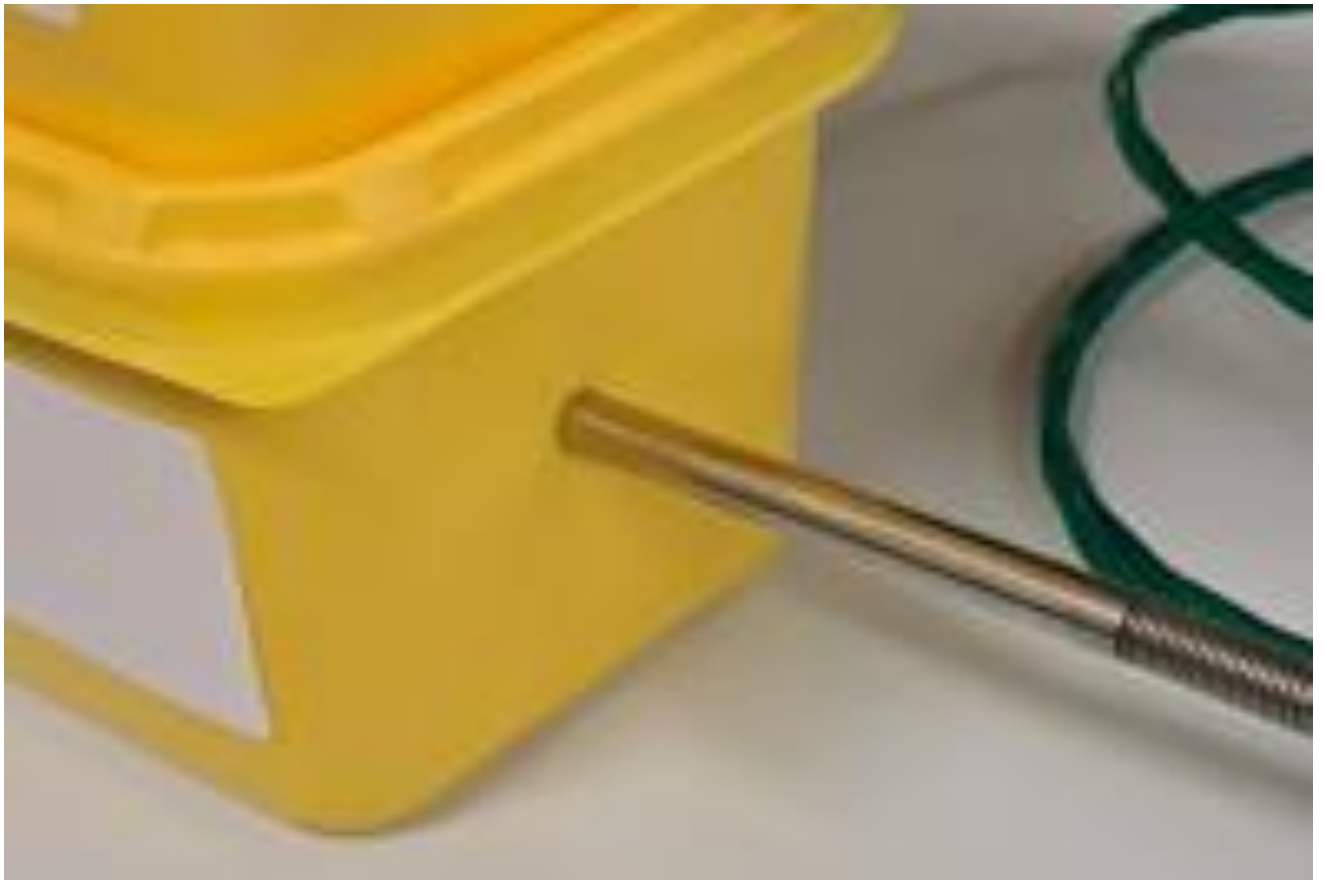
Figure 3.1. Photographic image of a temperature probe inserted in the side of temperature reference tub for one temperature treatment.
