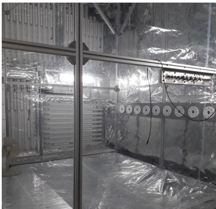
Figure 1.2 Photograph of the Irish atmospheric simulation chamber (IASC) at University College Cork, Ireland.
