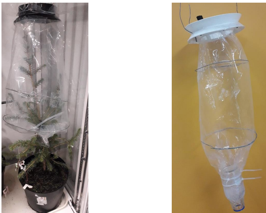
Figure 3.4 Enclosure around Spruce 3 (left), and Empty enclosure (right).
