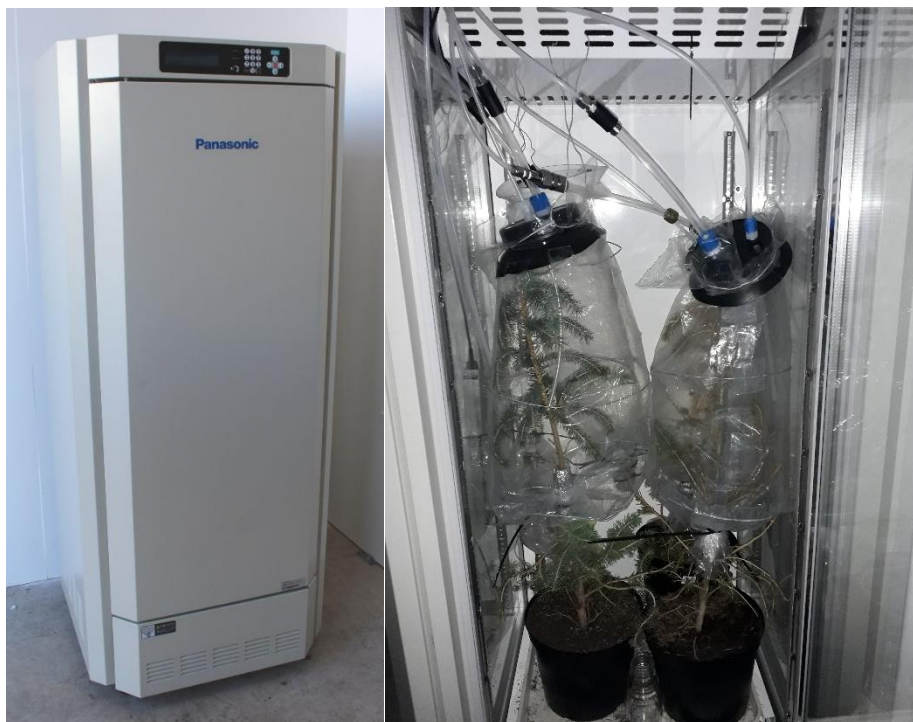
Figure 3.5 Plant growth chamber exterior (left) 159 , and interior with Spruce trees inside (right).
