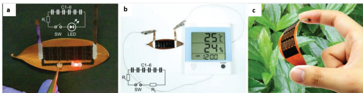
Figure 1.18 Fallen leaves gLIG electrodes used to power: a) LED, b) table clock; c) gLIG electrode on fallen leaf showing good flexibility. Readapted from [82], Copyright 2021, John Wiley and Sons.
