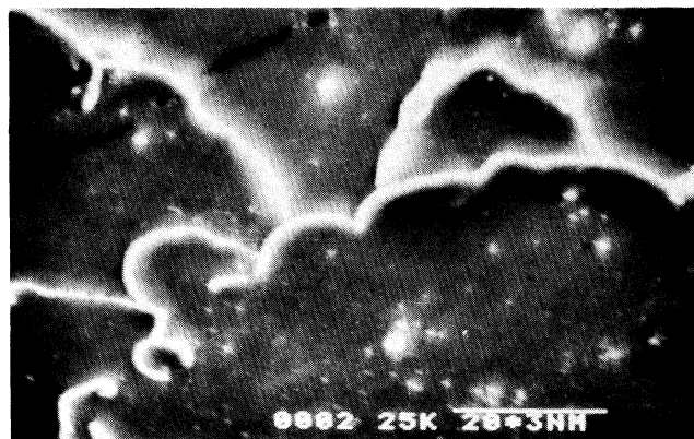
FIG. 11. Electron micrograph of silver deposit in glass F2 ion exchanged for 8 h \times 1500 .
