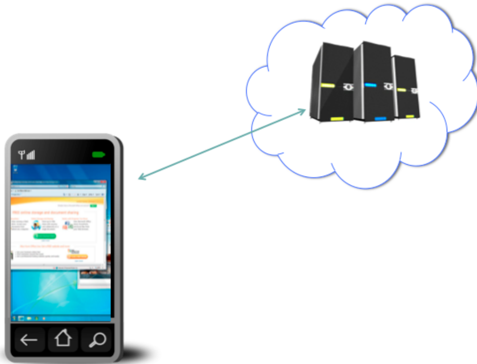
Figure 2.4: Remote Display Model. Similar to Cloudlets and application partitioning, a virtual machine runs on a cloud server. The component of the solution that displays the visual GUI output of the virtual machine runs on the mobile device.
